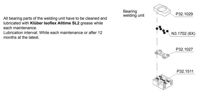
All other parts have to be greased due to the explosion drawing. Lubrication interval: While each maintenance
