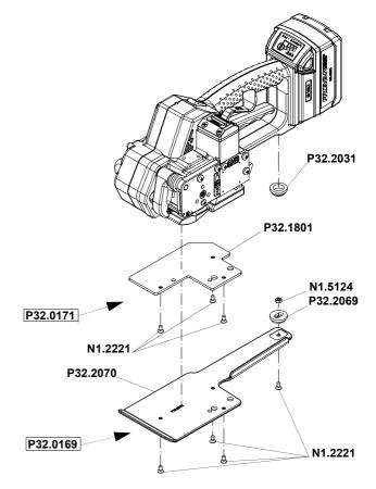
If the complete bottom side of the tool has to be protected, the plate P32.0169 must be used.
