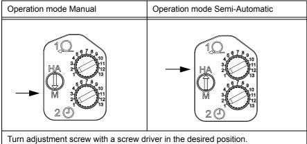
Turn adjustment screw with a screw driver in the desired position. Confirm the choice of the operation mode by pressing the tension button shortly.
